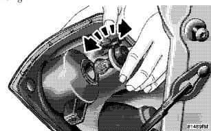
**Rotating Bulb Socket From Housing**
